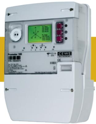
Prometer 100, series of next generation energy meter designed for power transfer points requiring precise measurements and revenue transactions. Flexible and modular communications ensure integration with AMR / AMI / SCADA systems and upgrade to future sub-station automation systems. 4 quadrant energy measurement allows monitoring of generation, transmission and distribution loads.
